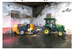
The sweeping unit of the MSH consists of two towed disc brushes with drive via the PTO of the tractor. The hydraulic lifting and lowering of the disc brushes can be controlled via the control panel. The MSH has a rear-mounted, collision-protected roller brush, while the adjustable roller brush cover ensures optimal sweeping results.
