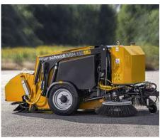
The MSH 150 has a steel hopper with 1.5  $\,\mathrm{m}^3$  capacity.
